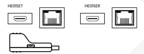
Connect a 5V power adapter via built-in micro USB at HE01SET when the source doesn't provide enough power to the receiver.
