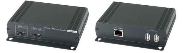
The HKM01E is design to extend full HDMI & USB keyboard mouse over one CAT5e/6 up to 150 meters. Transmitter built in local HDMI monitor output for local monitor and provides superior video quality up to 1920 x 1200 resolutions. With 2 USB port to extend keyboard and mouse signal over same CAT5e/6 cable. It is optimized for applications at security monitoring and multimedia display and digital signage, home network integration, and industrial control, hospital, education.
