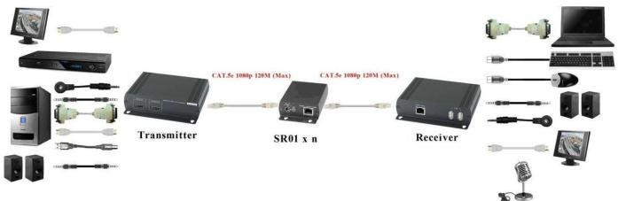
HDMI over IP Solution: support point to many connections via network switch:
